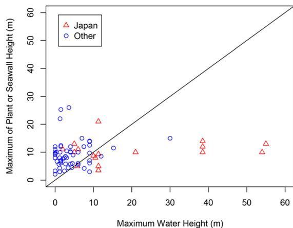
**Figure 2.** Maximum of plant or seawall height vs maximum water height.
