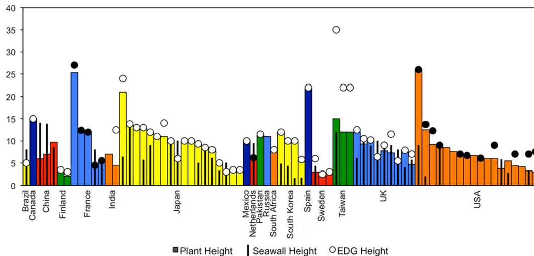
**Figure 1.** Plant, sea wall, and backup power height (m), international comparison. Note: Dark circles indicate waterproofing of EDG; open circles indicate no evidence of waterproofing. No circle indicates plant operator declined to release information on EDGs. No vertical bar indicates no sea wall.
