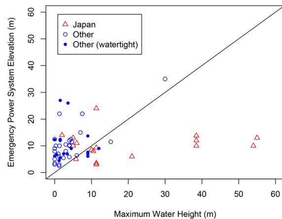
**Figure 3.** Emergency power system elevation vs maximum water height.
