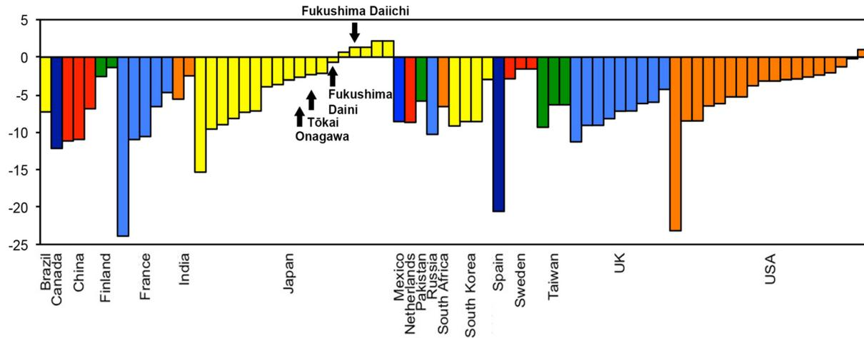
**Figure 4.** Difference of  $H_{av}$  and maximum of plant and sea wall height (m). Note: High numbers imply inadequate protection (i.e., high vulnerability to tsunami and low elevation of plant and sea wall). A number above zero means the plant and sea wall both lie below the average wave height of a historical incident.
